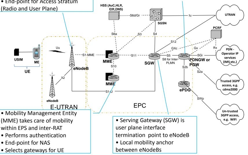
X2, S1-U, S2a, Rx etc. are reference points between network elements. Protocols are defined for each reference point. Solid lines between network elements are mainly for user plane traffic as defined by 3GPP while dashed lines are mainly for control plane.
